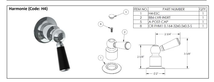
Specification from Finished Wall to Tip of Broach Stem
